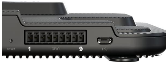
Figure 8: Impinj R700 Series GPIO Pin Locations
